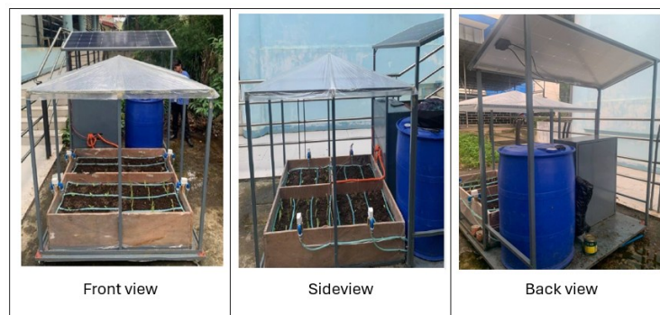
Figure 4. Fabricated multi-plot integrated prototype with control and irrigation subsystems
