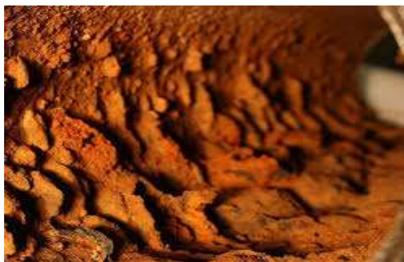
Figure 3. Microbiologically influenced corrosion
